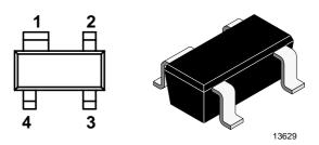
S595TXR Marking: X5R Plastic case (SOT 143R) 1 = Source, 2 = Drain, 3 = Gate 2, 4 = Gate 1
