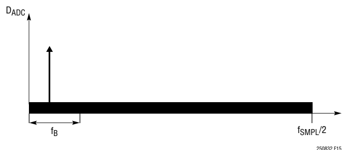
Figure 15. Frequency Spectrum of SAR ADC Core Output
