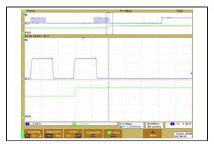
**FIGURE 2-16:**  $5 k\Omega - \text{Low-Voltage}$ Increment Wiper Settling Time  $(V_{DD} = 2.7V)$   $(1 \mu \text{s/Div})$ .
