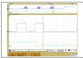
**FIGURE 2-34:** 50 k $\Omega$  – Low-Voltage Decrement Wiper Settling Time ( $V_{DD}$  = 5.5V) (1  $\mu$ s/Div).
