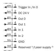
Do not connect for IVC-3D products with a type code as IVC-3Dxxx1x.
