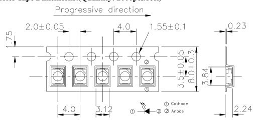
TOLERANCES UNLESS DIMENSION±0.1 ANGLE±0.5 UNIT: mm
