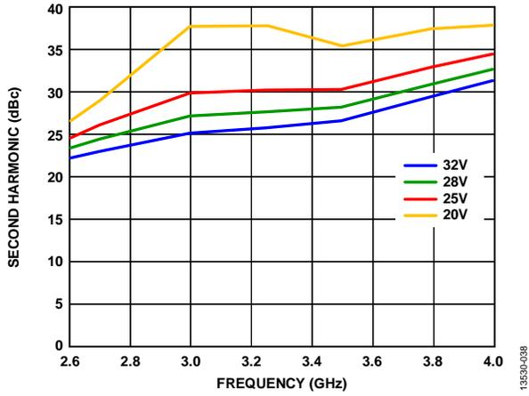
Figure 38. Second Harmonic vs. Frequency at Various Supply Voltages, P<sub>OUT</sub> = 30 dBm
