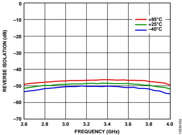
Figure 32. Reverse Isolation vs. Frequency at Various Temperatures
