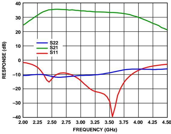
Figure 8. Response (Gain and Return Loss) vs. Frequency
