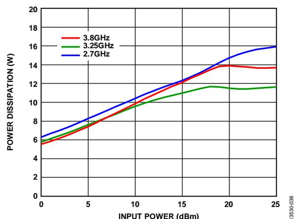
Figure 36. Power Dissipation vs. Input Power at 85°C
