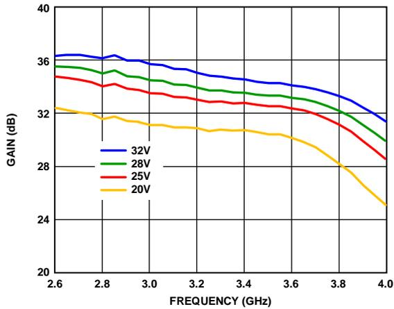
Figure 10. Gain vs. Frequency at Various Supply Voltages
