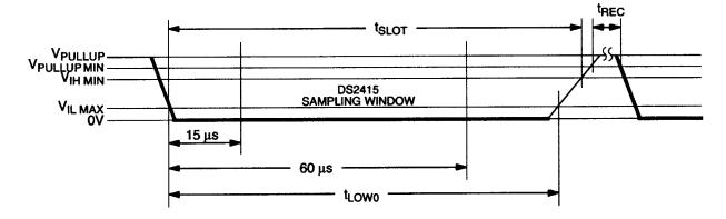
$$\begin{array}{l} 60\mu s \leq t_{LOW0} \leq t_{SLOT} \leq 120\mu s \\ 1\mu s \leq t_{REC} < \infty \end{array}$$
