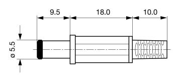
Cable diameter max. 4.0 mm
