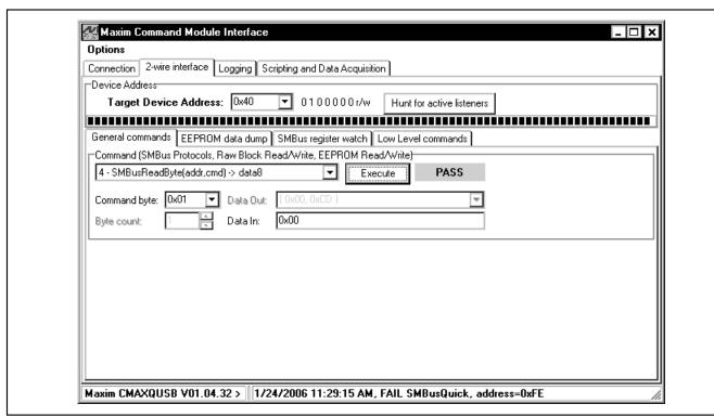
Figure 3. The 2-Wire Interface Window Provides Direct, Low-Level Access to the MAX6964 and 2-Wire Serial Interface
