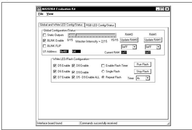
Figure 1. The MAX6964 Evaluation Kit Software Global and White LED Config/Status Main Window for Global Configuration, White LED and Flash Controls, and Software Status
