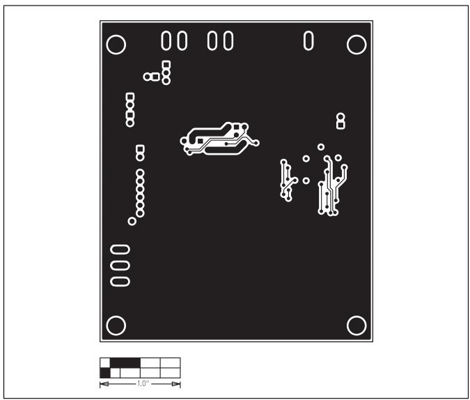
Figure 7. MAX6964 EV Kit PCB Layout—Solder Side
