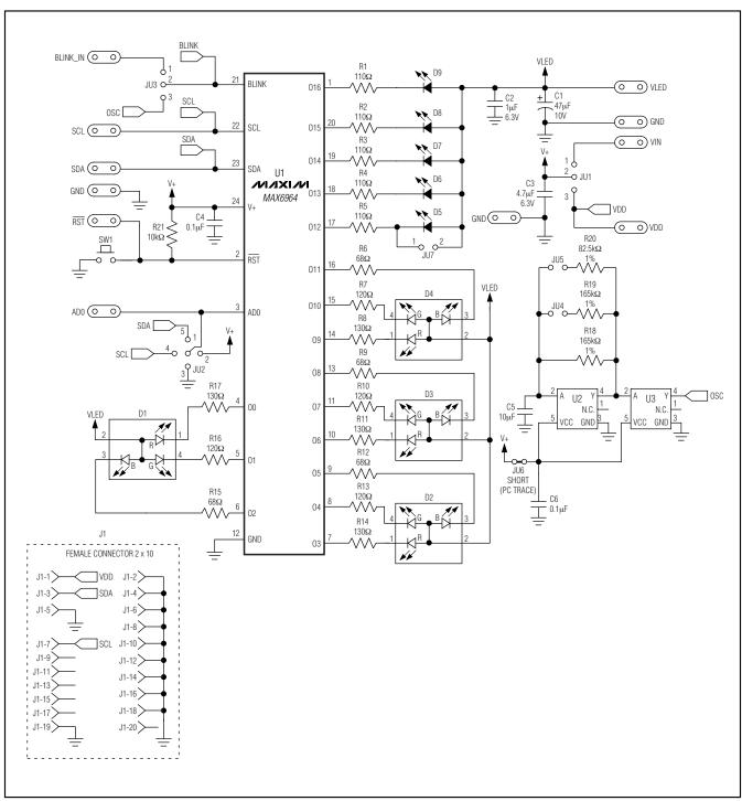
Figure 4. MAX6964 EV Kit Schematic
