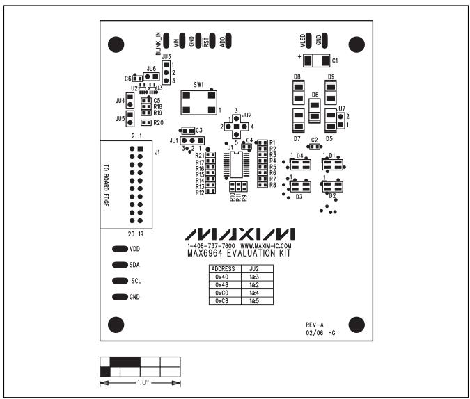
Figure 5. MAX6964 EV Kit Component Placement Guide—Component Side
