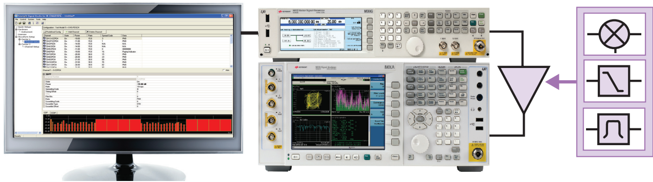
Figure 1. Typical component test configuration using Signal Studio's basic capabilities with a Keysight X-Series signal generator and an X-Series signal analyzer
