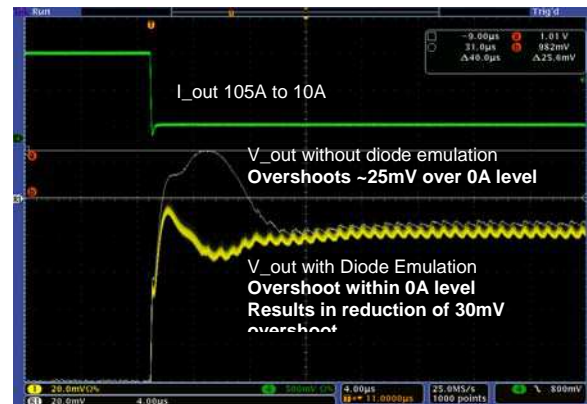
Figure 7: Output Voltage Overshoot Reduction with Diode Emulation
