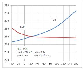
Figure 1: Ton and Toff (ns) Vs Temperature (°C)
