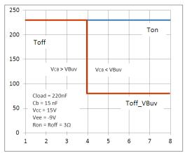
Figure 5: Ton, Toff (ns) Vs IN pulse duration (μs)
