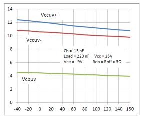
Figure 3: Vccuv+, Vccuv- and Vcbuv (V) Vs Temperature (°C)
