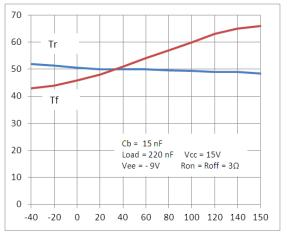
Figure 2: Tr and Tf (ns) Vs Temperature (°C)
