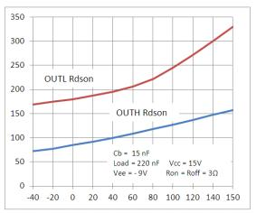
Figure 4: OUTH & OUTL Rdson's Vs Temperature (°C)
