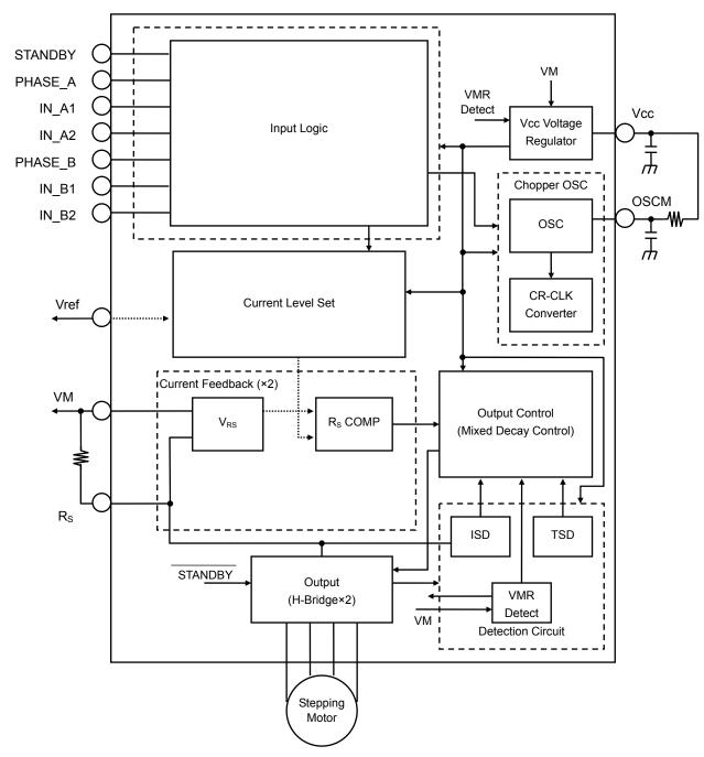
Note: All the grounding wires of the TB62218FG/FTG must run on the solder mask on the PCB and be externally terminated at only one point. Also, a grounding method should be considered for efficient heat dissipation.
