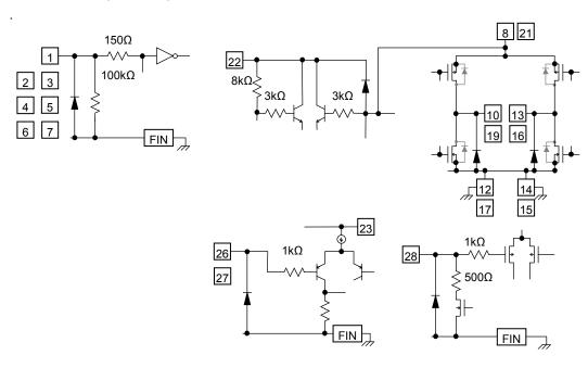
The equivalent circuit diagrams may be simplified or some parts of them may be omitted fo explanatory purposes. Absolute precision of the chip internal resistance is +/-30%.
