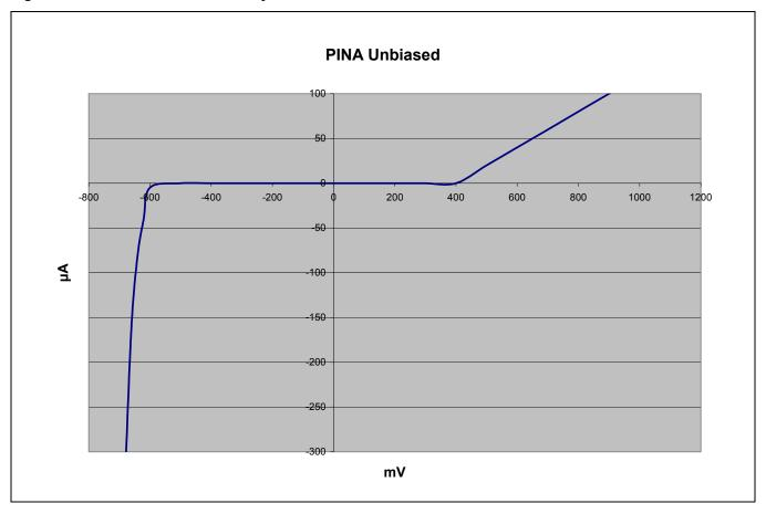
In the positive direction the impedance of the input is relatively high.
