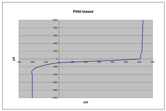
It can be seen that any negative voltage below 200 mV is nulled and that any positive going voltage above the PINA standing voltage is nulled by the DC servo. The DC servo upper bandwidth varies from part to part, but is generally at least 30 kHz.
