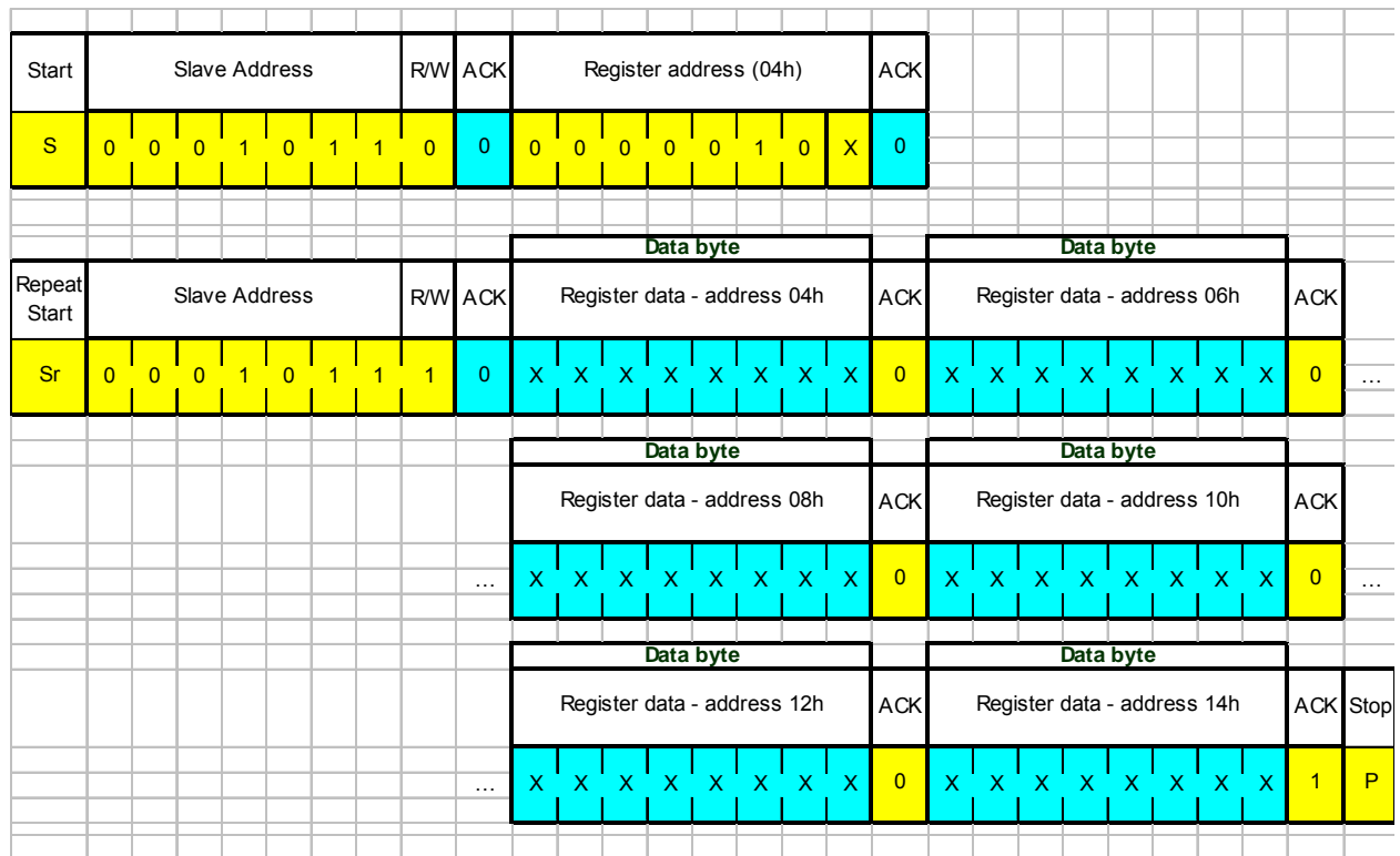
Figure 23: I 2 C multiple bytes read protocol
