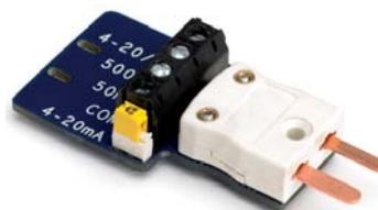
The PP624 is an optional terminal board for the TC-08. The screw terminals allow wires to be attached to the data logger without soldering and enable the TC-08 to measure voltages from 0 to +5 V, or 4-20 mA loop current.
