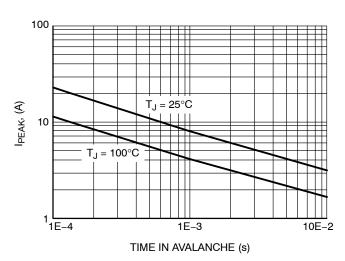
Figure 12. I<sub>PEAK</sub> vs. Time in Avalanche
