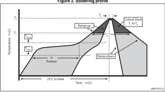
Figure 2. Soldering profile
