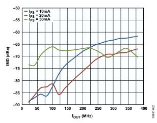
Figure 12. IMD vs.  $f_{OUT}$  over Full-Scale Current,  $4 \times$  Interpolation,  $f_{DATA} = 400$  MSPS, Digital Scale = 0 dBFS
