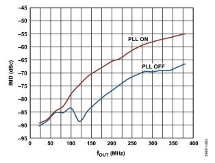
Figure 13. IMD vs.  $f_{OUT}$ ,  $4 \times$  Interpolation,  $f_{DATA} = 200$  MSPS, Digital Scale = 0 dBFS,  $I_{FS} = 20$  mA, PLL On and PLL Off
