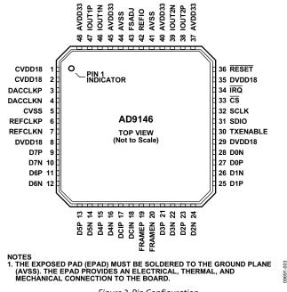
Figure 3. Pin Configuration
