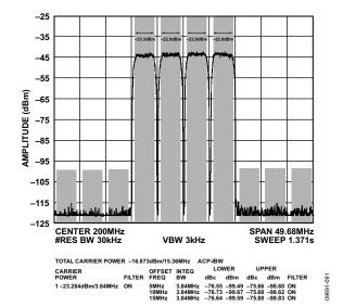
Figure 24. Four-Carrier W-CDMA Performance,  $4 \times$  Interpolation,  $f_{DATA} = 245.76$  MSPS, Digital Scale = -6 dBFS,  $f_{OUT} = 200$  MHz
