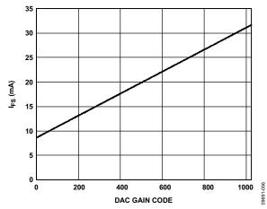
Figure 51. DAC Full-Scale Current vs. DAC Gain Code
