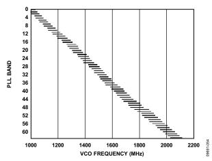
Figure 49. PLL Lock Range over Temperature for a Typical Device
