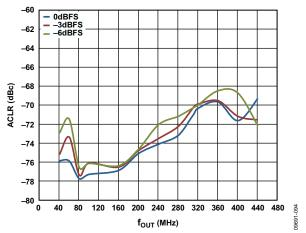
Figure 17. Four-Carrier W-CDMA ACLR vs. f<sub>OUT</sub> over Digital Scale, First Alternate Channel, 4× Interpolation, f<sub>DATA</sub> = 245.76 MSPS, PLL Off
