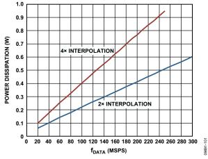
Figure 60. DVDD18 Power Dissipation vs.  $f_{DATA}$  Without Inverse Sinc
