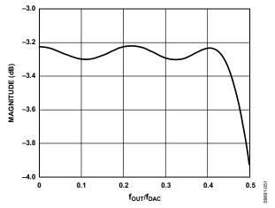
Figure 46. Sample Composite Responses of the Sinc<sup>-1</sup> Filter with sin(x)/x Roll-Off
