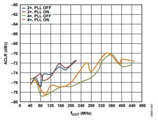
Figure 21. Four-Carrier W-CDMA ACLR vs. f<sub>OUT</sub> over Interpolation, Second Alternate Channel, f<sub>DATA</sub> = 245.76 MSPS, PLL Off and PLL On
