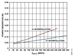
Figure 61. CVDD18 Power Dissipation vs. f<sub>DATA</sub> with PLL Disabled
