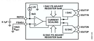
Figure 50. Simplified Block Diagram of DAC Core
