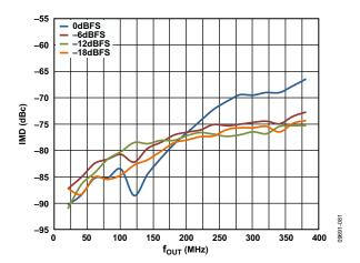
Figure 11. IMD vs.  $f_{OUT}$  over Digital Scale, 4× Interpolation,  $f_{DATA} = 400$  MSPS,  $I_{FS} = 20$  mA
