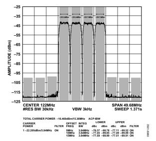
Figure 22. Four-Carrier W-CDMA Performance,  $4 \times$  Interpolation,  $f_{DATA} = 245.76$  MSPS, Digital Scale = -6 dBFS,  $f_{OUT} = 122$  MHz
