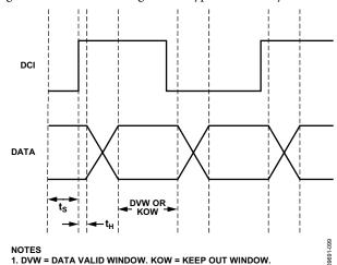
Figure 38. Timing Diagram for Input Data Port (Bypass DCI Delay Mode)
