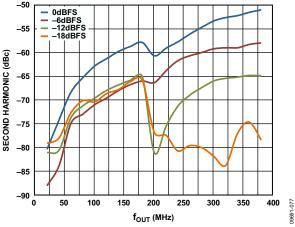
Figure 5. Second Harmonic vs.  $f_{OUT}$  over Digital Scale,  $4 \times$  Interpolation,  $f_{DATA} = 400$  MSPS,  $I_{FS} = 20$  mA
