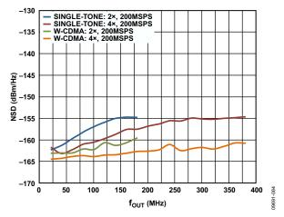
Figure 14. NSD vs.  $f_{OUT}$  over Interpolation, Single-Tone and W-CDMA Signals,  $f_{DATA} = 200$  MSPS, Digital Scale = 0 dBFS,  $I_{FS} = 20$  mA, PLL Off
