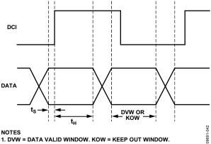
Figure 37. Timing Diagram for Input Data Port
