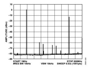
Figure 9. Single-Tone Spectrum,  $4 \times$  Interpolation,  $f_{DATA} = 200$  MSPS,  $f_{OUT} = 151$  MHz
