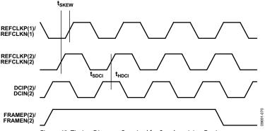
Figure 63. Timing Diagram Required for Synchronizing Devices
