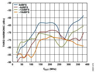
Figure 6. Third Harmonic vs.  $f_{OUT}$  over Digital Scale,  $4 \times$  Interpolation,  $f_{DATA} = 400$  MSPS,  $I_{FS} = 20$  mA
