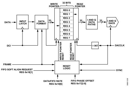
Figure 32. Block Diagram of FIFO
