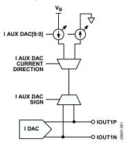
Figure 55. Auxiliary DAC Structure
