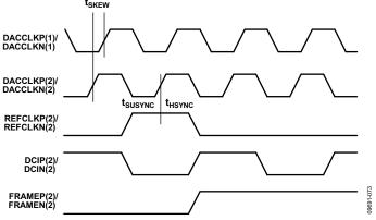
Figure 67. FIFO Rate Synchronization Signal Timing Requirements, 2× Interpolation
