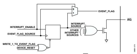
Figure 68. Simplified Schematic of IRQ Circuitry
