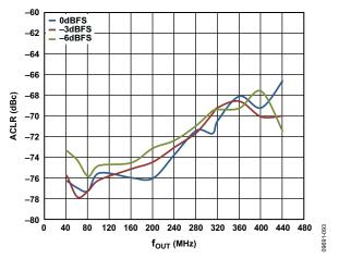
Figure 16. Four-Carrier W-CDMA ACLR vs.  $f_{OUT}$  over Digital Scale, Adjacent Channel,  $4 \times$  Interpolation,  $f_{DATA} = 245.76$  MSPS, PLL Off
