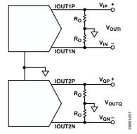
Figure 52. Basic Transmit DAC Output Circuit
