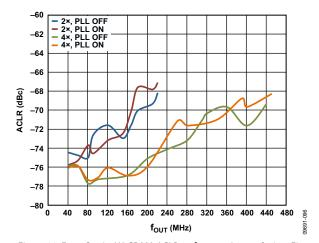
Figure 20. Four-Carrier W-CDMA ACLR vs. f<sub>OUT</sub> over Interpolation, First Alternate Channel, f<sub>DATA</sub> = 245.76 MSPS, PLL Off and PLL On
