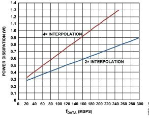
Figure 59. Total Power Dissipation vs.  $f_{DATA}$  Without PLL and Inverse Sinc
