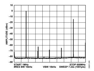
Figure 8. Single-Tone Spectrum,  $2 \times$  Interpolation,  $f_{DATA} = 300$  MSPS,  $f_{OUT} = 101$  MHz
