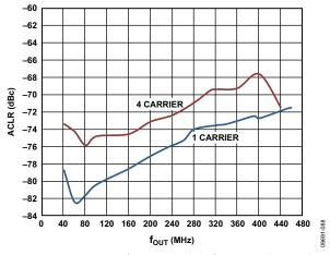
Figure 23. W-CDMA ACLR vs.  $f_{OUT}$  over Number of Carriers, Adjacent Channel, 4× Interpolation,  $f_{DATA}$  = 245.76 MSPS, Digital Scale = -6 dBFS, PLL Off
