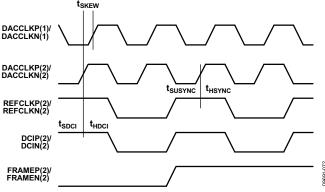
Figure 65. Data Rate Synchronization Signal Timing Requirements, 2× Interpolation
