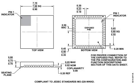
Figure 70. 48-Lead Lead Frame Chip Scale Package [LFCSP\_WQ] 7 mm × 7 mm Body, Very Very Thin Quad (CP-48-13) Dimensions shown in millimeters
