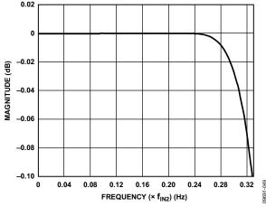
Figure 44. Pass-Band Detail of HB2
