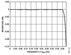
Figure 41. Pass-Band Detail of HB1
