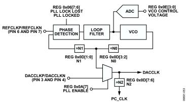
Figure 48. PLL Clock Multiplication Circuit
