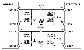
Figure 57. Passive, Level-Shifting Network for Biasing the ADL5375-15
