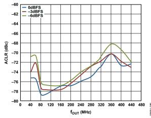
Figure 18. Four-Carrier W-CDMA ACLR vs.  $f_{OUT}$  over Digital Scale, Second Alternate Channel,  $4 \times$  Interpolation,  $f_{DATA} = 245.76$  MSPS, PLL Off
