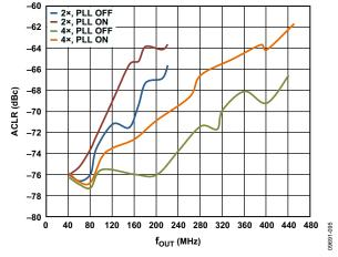
Figure 19. Four-Carrier W-CDMA ACLR vs. f<sub>OUT</sub> over Interpolation, Adjacent Channel, f<sub>DATA</sub> = 245.76 MSPS, PLL Off and PLL On
