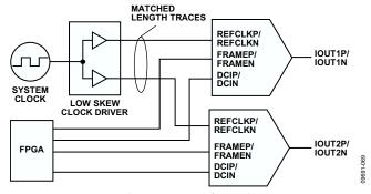
Figure 62. Typical Circuit Diagram for Synchronizing Devices
