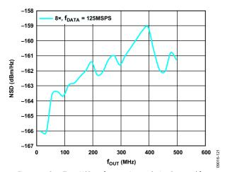
Figure 24. One-Tone NSD vs.  $f_{OUT}$  over Interpolation Rate and  $f_{DATA}$ , Digital Scale = 0 dBFS,  $f_{SC}$  = 20 mA, PLL On
