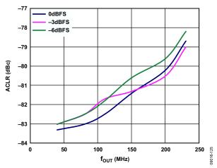
Figure 28. One-Carrier W-CDMA ACLR vs. f<sub>OUT</sub> over Digital Cutback, Adjacent Channel, PLL Off
