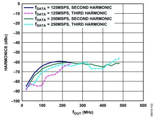
Figure 5. Harmonics vs.  $f_{OUT}$  over  $f_{DATA}$ ,  $4\times$  Interpolation, Digital Scale = 0 dBFS,  $f_{SC}$  = 20 mA
