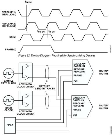
Figure 83. Typical Circuit Diagram for Synchronizing Devices to a System Clock
