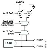
Figure 72. Auxiliary DAC Structure
