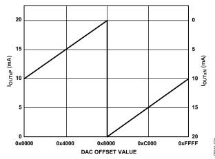
Figure 61. DAC Output Currents vs. DAC Offset Value
