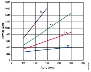
Figure 76. Total Power Dissipation vs. f<sub>DATA</sub> Without PLL, Fine NCO, and Inverse Sinc
