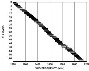
Figure 65. PLL Lock Range over Temperature for a Typical Device
