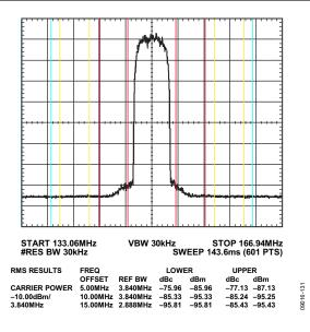
Figure 34. Four-Carrier W-CDMA ACLR Performance, IF ≈150 MHz
