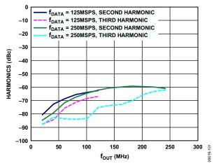
Figure 4. Harmonics vs.  $f_{OUT}$  over  $f_{DATA}$ , 2× Interpolation, Digital Scale = 0 dBFS,  $f_{SC}$  = 20 mA
