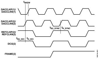
Figure 84. Data Rate Synchronization Signal Timing Requirements, 2× Interpolation
