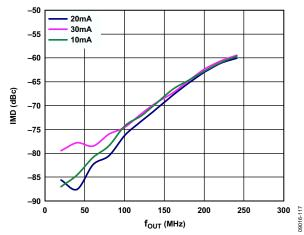
Figure 20. IMD vs.  $f_{OUT}$  over  $f_{SC}$ ,  $2 \times$  Interpolation,  $f_{DATA} = 250$  MSPS, Digital Scale = 0 dBFS
