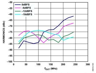
Figure 8. Third Harmonic vs.  $f_{OUT}$  over Digital Scale, 2× Interpolation,  $f_{DATA} = 250$  MSPS,  $f_{SC} = 20$  mA
