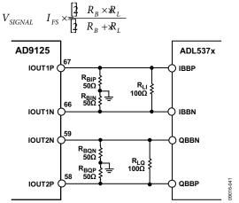
Figure 73. Typical Interface Circuitry Between the AD9125 and the ADL537x Family of Modulators
