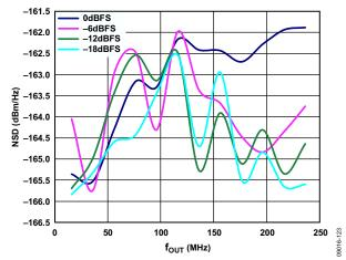
Figure 26. Eight-Tone NSD vs.  $f_{OUT}$  over Digital Scale,  $f_{DATA} = 200$  MSPS,  $4 \times$  Interpolation,  $f_{SC} = 20$  mA, PLL Off
