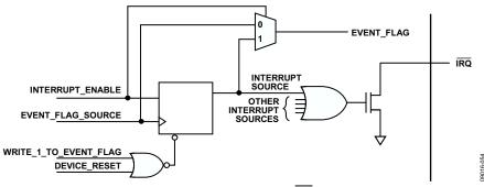
Figure 86. Simplified Schematic of IRQ Circuitry
