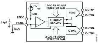
Figure 66. Simplified Block Diagram of DAC Core
