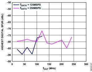
Figure 10. Highest Digital Spur vs.  $f_{OUT}$  over  $f_{DATA}$ ,  $2\times$  Interpolation, Digital Scale = 0 dBFS,  $f_{SC}$  = 20 mA
