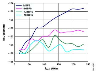
Figure 23. One-Tone NSD vs.  $f_{OUT}$  over Digital Scale,  $f_{DATA} = 200$  MSPS,  $4 \times$  Interpolation,  $f_{SC} = 20$  mA, PLL Off
