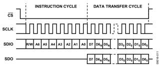
Figure 38. Serial Register Interface Timing, MSB First
