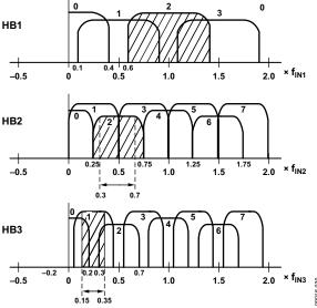
Figure 60. Signal Propagation for 8× Interpolation (f<sub>DATA</sub> Modulation)
