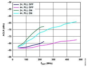
Figure 31. One-Carrier W-CDMA ACLR vs. f<sub>OUT</sub> over Interpolation Rate, Adjacent Channel, PLL On vs. PLL Off
