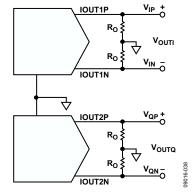
Figure 68. Basic Transmit DAC Output Circuit
