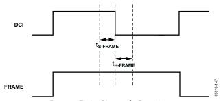
Figure 46. Timing Diagram for Frame input
