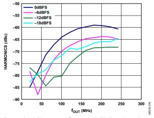
Figure 7. Second Harmonic vs.  $f_{OUT}$  over Digital Scale,  $2 \times$  Interpolation,  $f_{DATA} = 250$  MSPS,  $f_{SC} = 20$  mA
