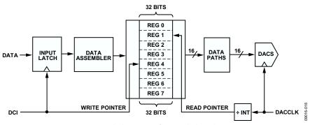
Figure 47. Block Diagram of Datapath Through FIFO
