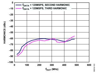
Figure 6. Harmonics vs.  $f_{OUT}$  over  $f_{DATA}$ , 8× Interpolation, Digital Scale = 0 dBFS,  $f_{SC}$  = 20 mA
