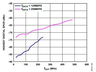
Figure 11. Highest Digital Spur vs.  $f_{OUT}$  over  $f_{DATA}$ ,  $4 \times$  Interpolation, Digital Scale = 0 dBFS,  $f_{SC}$  = 20 mA
