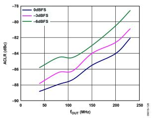
Figure 29. One-Carrier W-CDMA ACLR vs. f<sub>OUT</sub> over f<sub>DAC</sub>, Alternate Channel, PLL Off
