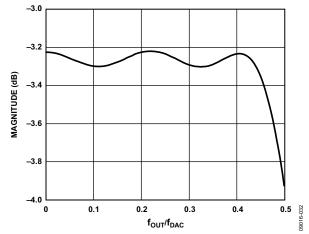
Figure 62. Sample Composite Responses of the Sinc<sup>-1</sup> Filter with Sin(x)/x Roll-Off
