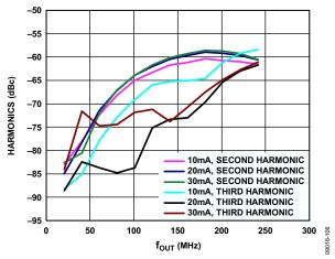
Figure 9. Harmonics vs.  $f_{OUT}$  over  $f_{SC}$ , 2× Interpolation,  $f_{DATA} = 250$  MSPS, Digital Scale = 0 dBFS
