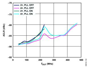
Figure 33. One-Carrier W-CDMA ACLR vs.  $f_{\text{OUT}}$  over Interpolation Rate, Second Alternate Channel, PLL On vs. PLL Off
