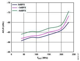
Figure 30. One-Carrier W-CDMA ACLR vs. f<sub>OUT</sub> over f<sub>DAC</sub>, Second Alternate Channel, PLL Off
