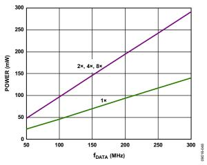
Figure 80. DVDD18 Power Dissipation vs. f<sub>DATA</sub> Due to Fine NCO
