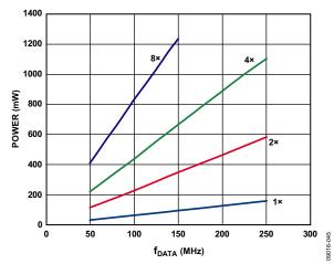
Figure 77. DVDD18 Power Dissipation vs. f<sub>DATA</sub> Without Fine NCO and Inverse Sinc
