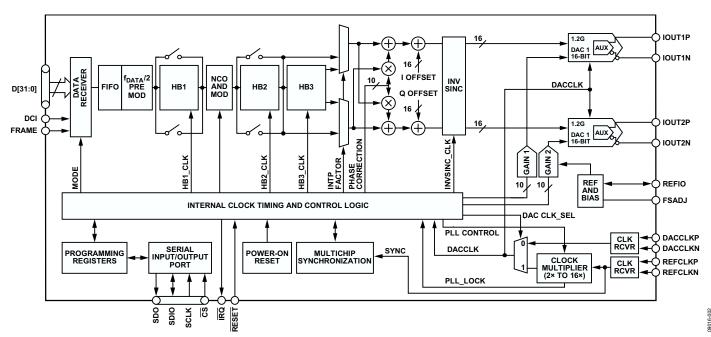
Figure 2. AD9125 Functional Block Diagram
