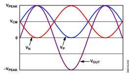
Figure 69. Voltage Output Waveforms
