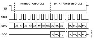
Figure 39. Serial Register Interface Timing, LSB First
