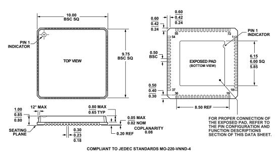
Figure 89. 72-Lead Lead Frame Chip Scale Package [LFCSP\_VQ] 10 mm × 10 mm Body, Very Thin Quad (CP-72-7) Dimensions shown in millimeters
