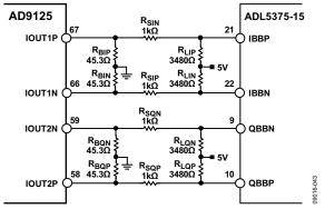
Figure 74. Passive Level-Shifting Network for Biasing ADL5375-15
