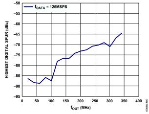
Figure 12. Highest Digital Spur vs.  $f_{OUT}$  over  $f_{DATA}$ , 8× Interpolation, Digital Scale = 0 dBFS,  $f_{SC}$  = 20 mA
