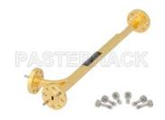
WR-12 10 dB Directional Waveguide Coupler With UG-387/U Flange and E-Plane Coupled Port From 60 GHz to 90 GHz E Band
