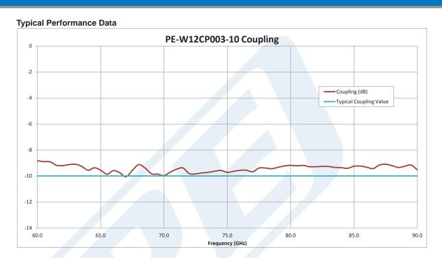
Click the following link (or enter part number in "SEARCH" on website) to obtain additional part information including price, inventory and certifications: WR-12 10 dB Directional Waveguide Coupler With UG-387/U Flange and E-Plane Coupled Port From 60 GHz to 90 GHz E Band PE-W12CP003-10
