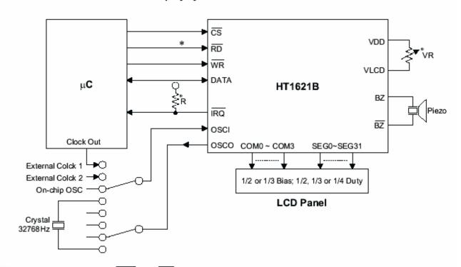
Note: The connection of  $\overline{IRQ}$  and  $\overline{RD}$  pin can be selected depending on the requirement of the  $\mu C$ .
