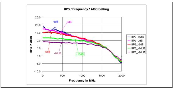
Figure 30 - Typical IIP3 @ Max Gain Differential / Frequency
