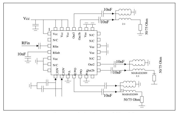
Figure 3 - Application Diagram - A (Differential)
