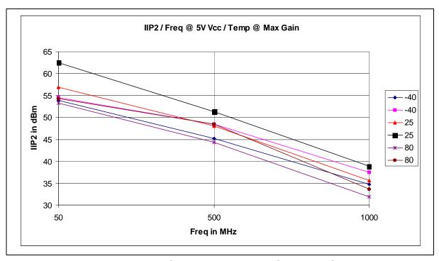
Figure 21 - Typical Out1 @ Out2 IIP2 / Frequency @ Max Gain @ 5V Vcc / Temp
