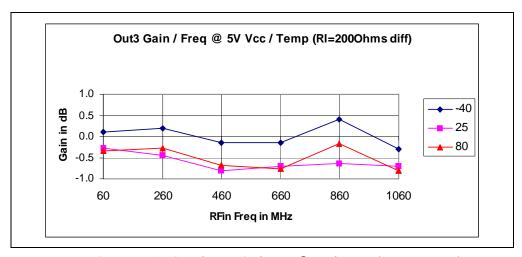
Figure 9 - Typical Ch3 Gain / Freq @ 5V / Temp (R1=200 Ohm)
