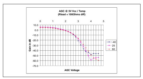
Figure 13 - Typical AGC / Temp @ 5 V Vcc
