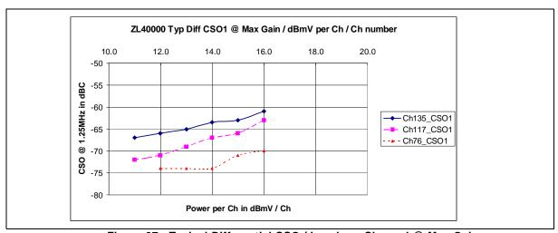
Figure 37 - Typical Differential CSO / Level per Channel @ Max Gain
