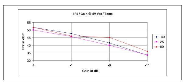
Figure 23 - Typical IIP2 / Gain @ 5V Vcc / Temp @ 500MHz
