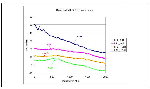
Figure 25 - Typical Single Ended IIP2 / Frequency / AGC
