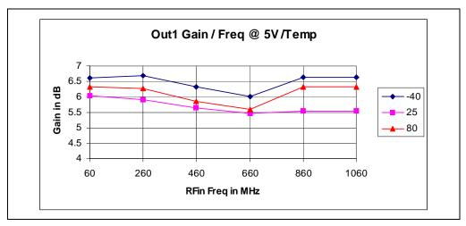
Figure 8 - Typical Ch1 & Ch2 Diff Max Gain / Freq / Temp @ 5V Vcc
