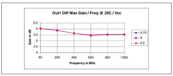
Figure 6 - Typical Ch1&2 Diff Gain / Freq / Vcc @ 25C
