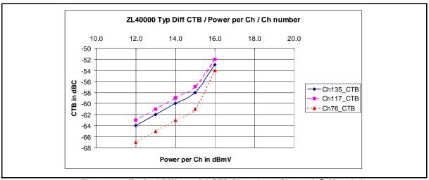
Figure 38 - Typical Differential CTB / Level per Channel @ Max Gain
