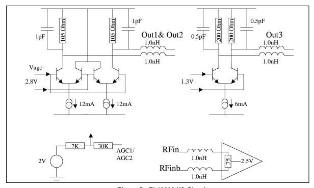
Figure 5 - ZL40000 I/O Circuits
