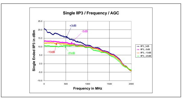
Figure 31 - Typical IIP3 Single Ended / Frequency / AGC
