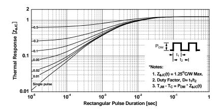
Figure 14. Transient Thermal Response Curve -FDPF5N60NZ
