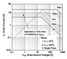
Figure 11. Maximum Drain Current vs.
