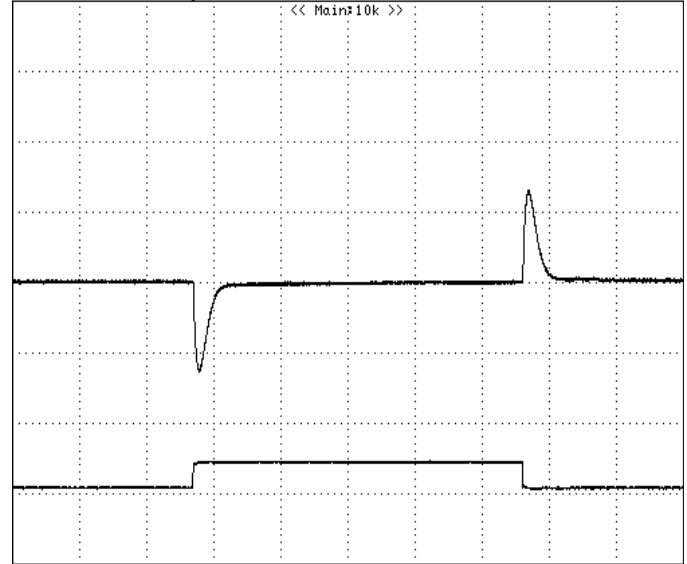
Figure 9: Output voltage response to step-change in load current (75%-50%-75% of I_o , max; di/dt = 2.0A/\mu s ). Load cap: 330\mu F , 35m\Omega ESR solid electrolytic capacitor and 1\mu F ceramic capacitor. Top Trace: V_{out} (100mV/div, 500us/div), Bottom Trace: I_{out} (2A/div). Scope measurement should be made using a BNC cable (length shorter than 20 inches). Position the load between 51 mm to 76 mm (2 inches to 3 inches) from the module.
