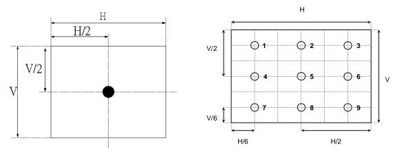
Fig.4-2 Optical measurement point
