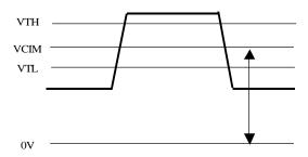
Figure: LVDS Differential Voltage
