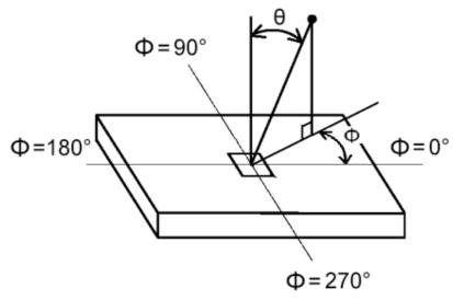
Fig.4-4 Viewing angle definition
