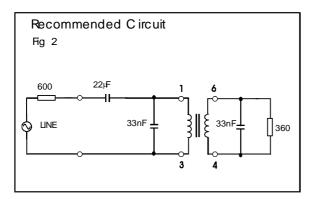
In p ractice the 360  $\Omega$  lo ad r esistor in fig ure 2 will connect to a low output impedance TX driver. The 33nF capacitor on the load side should appear in parallel w ith the 360  $\Omega$  r esistor (ra ther th an in parallel with the transformer winding) to obtain flat TX response to line.
