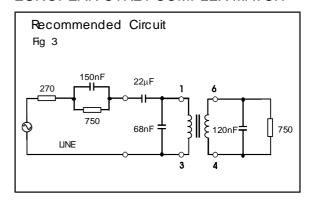
In practice, the  $750\Omega$  load resistor will connect to a low output impedance TX driver. The 120nF capacitor, which should have a temperature stable dielectric, should appear in parallel with the  $750\Omega$  resistor (rather than in parallel with the transformer winding) to obtain flat TX response to line.
