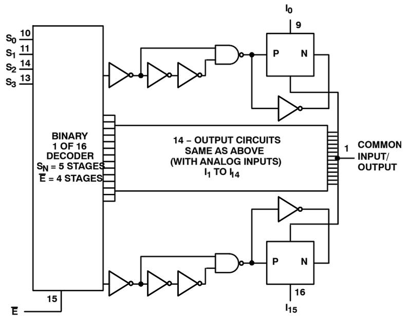
Figure 2. Function Diagram
