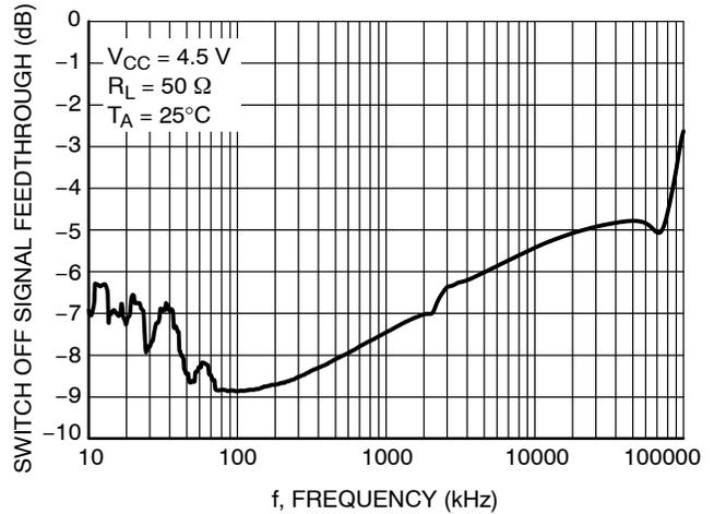
Figure 6. Typical Switch OFF Signal Feedthrough vs Frequency
