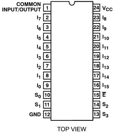
Figure 1. Pin Assignment
