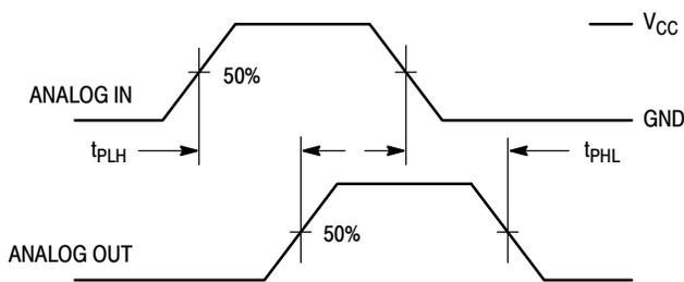
Figure 10. Propagation Delay, Analog In to Analog Out
