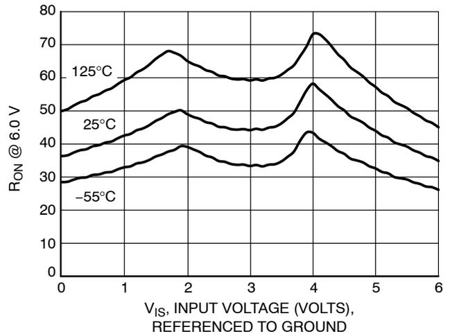
Figure 4. Typical On Resistance,  $V_{CC} = 6.0\text{ V}$
