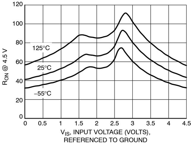
Figure 3. Typical On Resistance,  $V_{CC} = 4.5\text{ V}$
