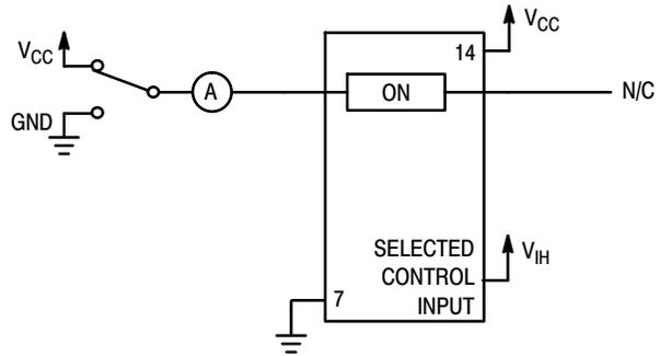
Figure 9. ON Channel Leakage Current Test Setup
