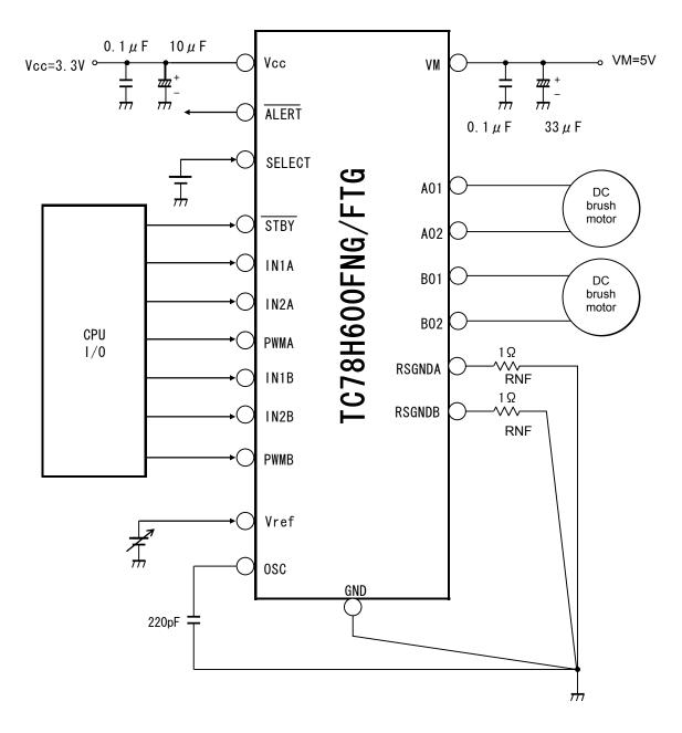
Note 1: A power supply capacitor should be connected as close as possible to the IC.
