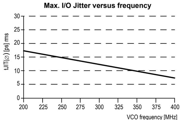
**Figure 4. Maximum I/O Jitter (RMS) versus frequency for  $V_{CC}=3.3V$**
