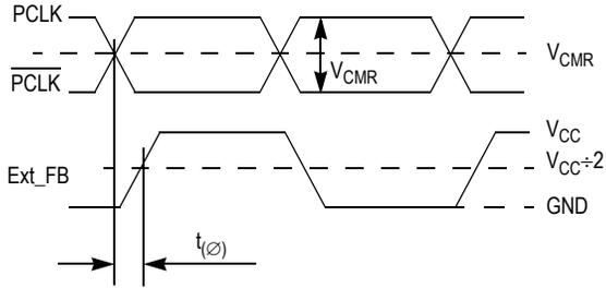
Figure 11. Propagation delay ( $t_{PD}$ , static phase offset) test reference
