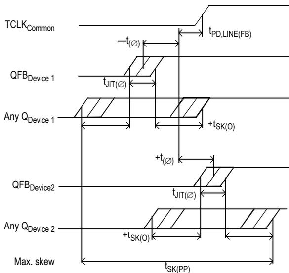
**Figure 3. MPC93H51 maximum device-to-device skew**
