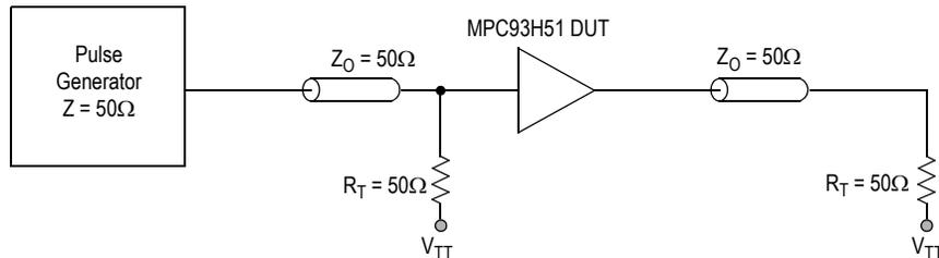
Figure 9. TCLK MPC93H51 AC test reference for V<sub>CC</sub> = 3.3V
