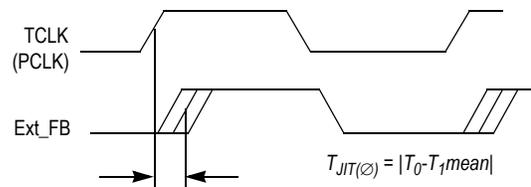
The deviation in  $t_0$  for a controlled edge with respect to a  $t_0$  mean in a random sample of cycles
