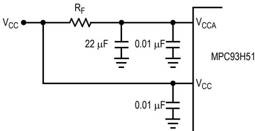
**Figure 5.  $V_{CCA}$  Power Supply Filter**
