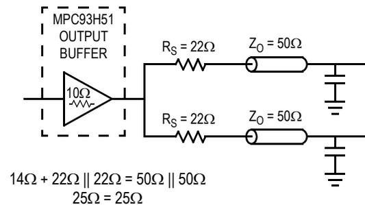
Figure 8. Optimized Dual Line Termination
