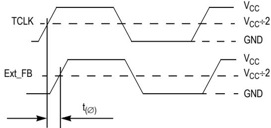
Figure 12. Propagation delay ( $t_{PD}$ ) test reference
