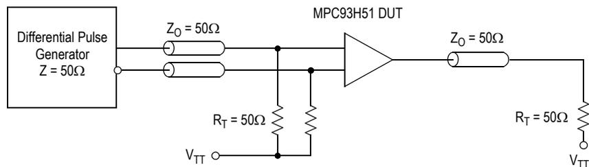
Figure 10. PCLK MPC93H51 AC test reference
