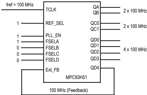
**MPC93H51 zero-delay configuration (feedback of QD4)**
