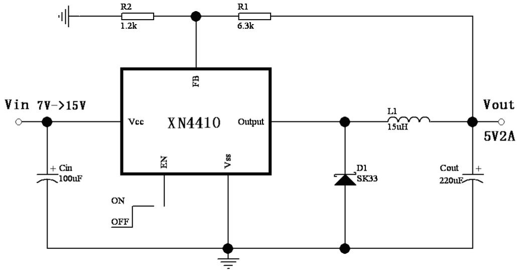
注意:  $V_{OUT} = V_{FB} \times (1 + R_1/R_2)$ ,  $R_2 = 0.7K \sim 5K \text{ ohm}$
