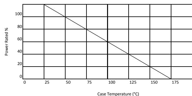
The case temperature is to be used for the definition of the applied power limit
