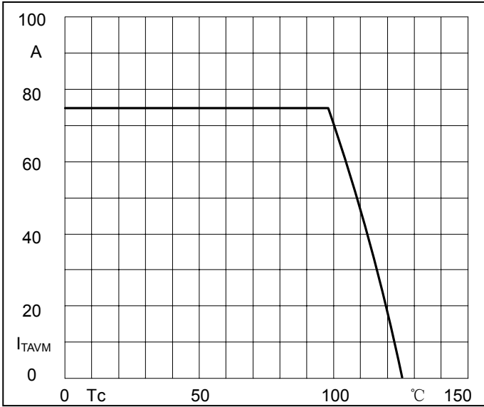
Fig7. SCR Forward Current Derating Curve
