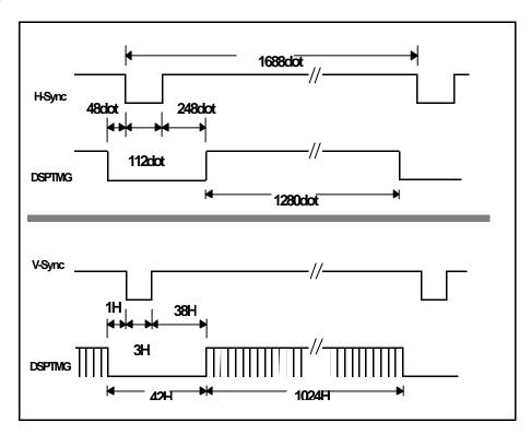
Note :1280X1024 at 75 Hz (VESA STANDARD), Horizontal line rate :13.02us, Dot clock :135MHz.
