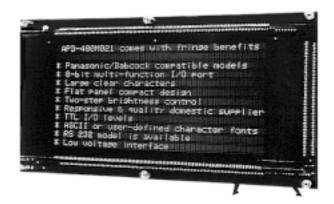
The APD-480M021 display module displays up to 480 alphanumeric 5 x 7 dot matrix characters arranged in 12 lines of 40 characters each.
