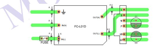
$\label{eq:Figure 4: EMC application circuit PCB layout Safety and recommend wiring: linewidth A {\geqslant} 3mm, C {\geqslant} 9mm$
