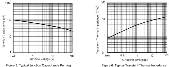
Figure 6. Typical Transient Thermal Impedance
