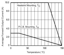
Figure 1. Derating Curve Output Rectified Current
