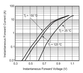
Figure 3. Typical Forward Characteristics Per Leg
