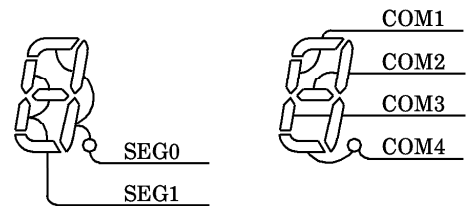
Figure 3-16. Example of COM and SEG connections
