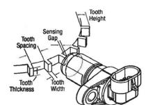
For best results, we recommend targets made from low carbon cold rolled steel. Other factors that influence sensor performance include geartooth height and width, space between teeth, shape of the teeth and thickness of the target. As a general guideline, consider a target with the following minimum parameters:
