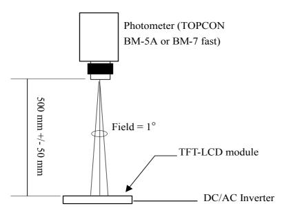
Optical characteristics measuring configuration
