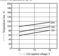
1-(2). Coil temperature rise (at 85°C 185°F) Sample: ACJ1212, 3pcs Measured portion: Inside the coil Contact carrying current: 10A, 15A, 20A Ambient temperature: 85°C 185°F
