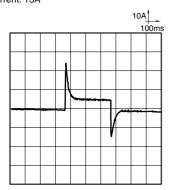
2-(2). Electrical life test (Motor lock)
