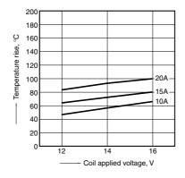
1-(3). Coil temperature rise (at room temperature)
