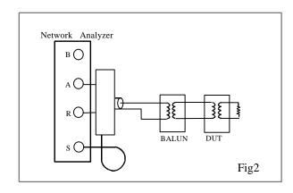
Return loss measure the amount of energy that is lost due to Reflection.
