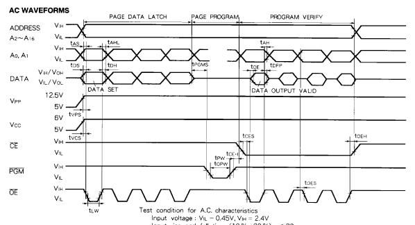
Input rise and fall time (10 %~90 %) :  $\leq$  20ns Reference voltage at timing measurement : Input, Output "L" = 0.8V, "H" = 2V
