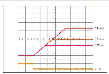
Figure 8: Turn-on transient with 24 V input; zero load (20 ms/div). ON/OFF input (5V/div) Ch 1-3: Vout (10V/div)
