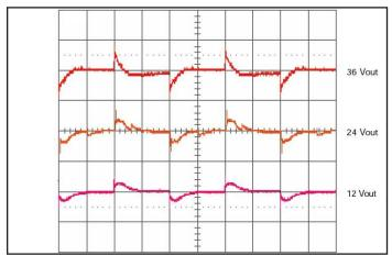
Figure 11: Output voltage response for 24V input; 12V, 24V, 36V output to step-change in load current (50-75-50% of Iout max; di/dt=0.1 $A/\mu$ s). Load cap:  $100\mu$ F,  $100m\Omega$  ESR tant, Ch 1-3: Vout (2V/div); (5ms/div).
