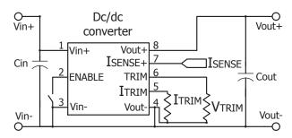
Figure C: Current monitor/trimmable current limit setup
