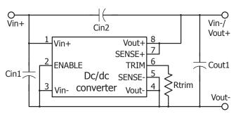
Figure B: Negative output setup
