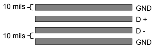
Figure 11. Recommended Remote Diode Circuit Board Interconnect
