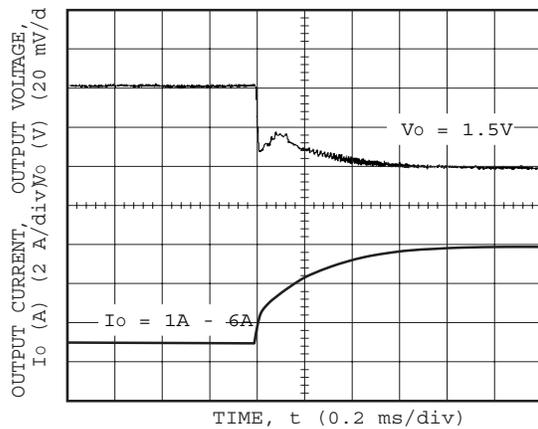
Figure 22. Transient Response Characteristic of 3.3VIN/1.5VOUT with IOUT step up 1A-6A Static load.
