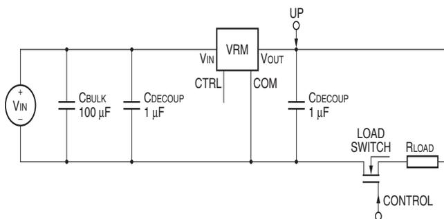
Figure 45. Load Transient Circuit.
