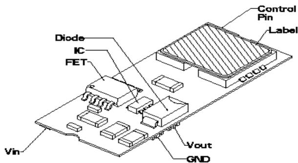
Figure 48. Temperature Measurement Location.
