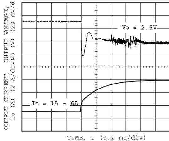
**Figure 28.** Transient Response Characteristic of 3.3VIN/ 2.5VOUT with IOUT step up 1A-6A Static load.
