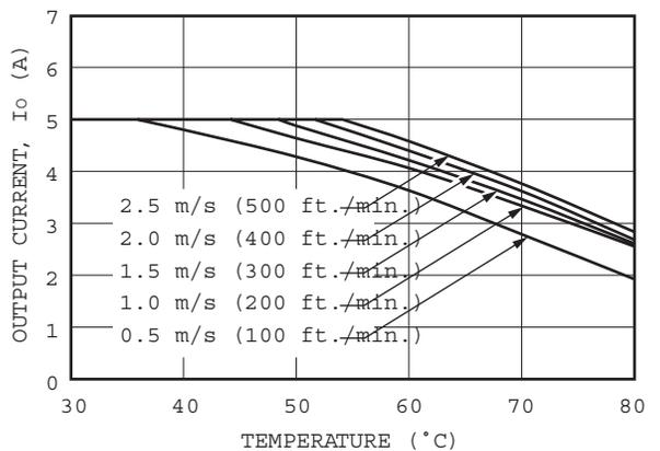
Figure 41. Thermal Derating for 5.0VIN ,2.0VOUT.
