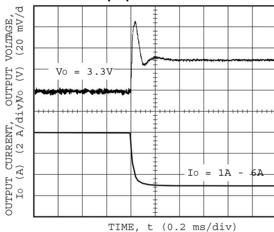
**Figure 35. Transient Response Characteristic of 5.0VIN/3.3VOUT with IOU step up 6A-1A Static load.**
