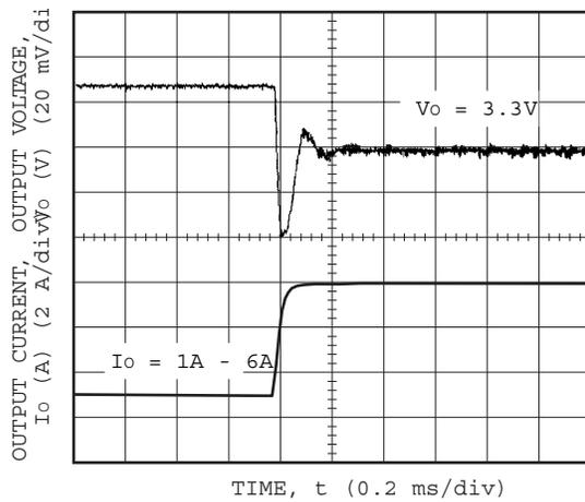
**Figure 34. Transient Response Characteristic of 5.0VIN/3.3VOUT with IOU step up 1A-6A Static load.**
