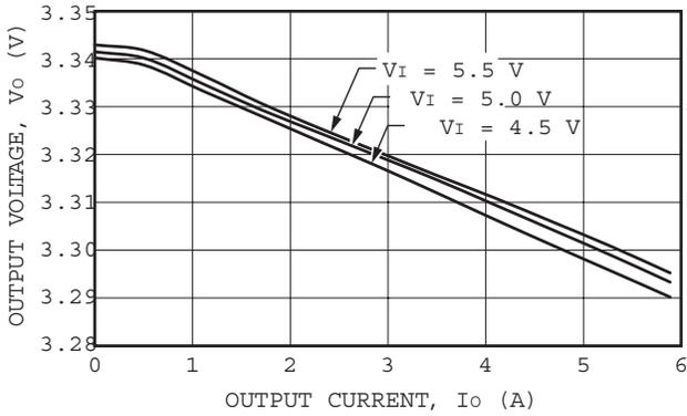
**Figure 21. Stactic Regulation: 5.0VIN,3.3VOUT.**
