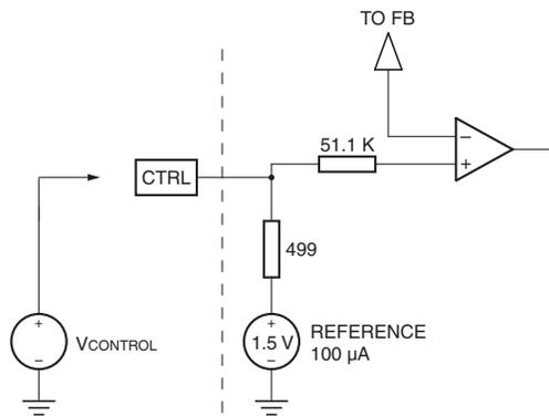
Figure 46. Circuit for increasing the output voltage.
