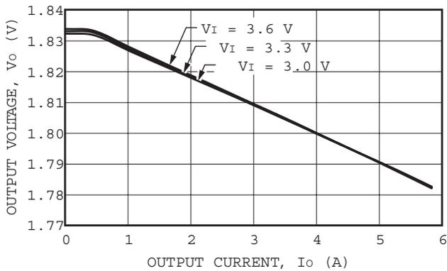
Figure 16. Static Regulation 3.3VIN,1.8VOUT.
