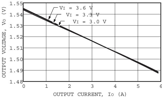
Figure 15. Static Regulation: 3.3VIN,1.5VOUT.
