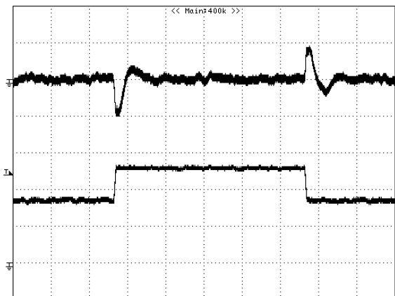
Figure 9: Output voltage response to step-change in load current (75%-50%-75% of I_{o, max} ; di/dt = 1.0A/\mu s ). Load cap: 2000 \mu F tantalum capacitor and 1 \mu F ceramic capacitor. Top Trace: V_{out} (50mV/div, 200us/div), Bottom Trace: I_{out} (10A/div). Scope measurement should be made using a BNC cable (length shorter than 20 inches). Position the load between 51 mm to 76 mm (2 inches to 3 inches) from the module
