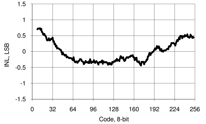
Figure 11-42. IDAC INL vs Input Code, Range = 255 \mu A, Sink Mode
