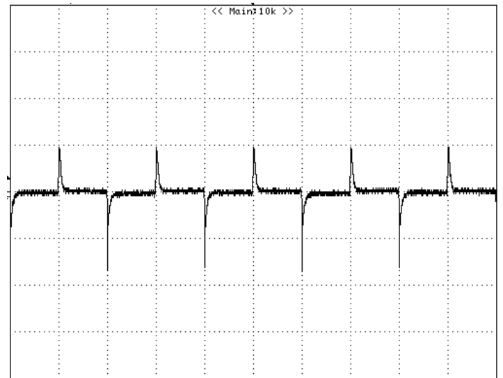
Figure 20: Typical transient response to step load change at 1A/\mu S from 100%~ 0%~100% of I_o , max at 12Vin, 0.59Vout (Cout = 1uF ceramic, 47uF+10uFceramic) CH1 : VOUT, 0.1V/div, 5mS/div
