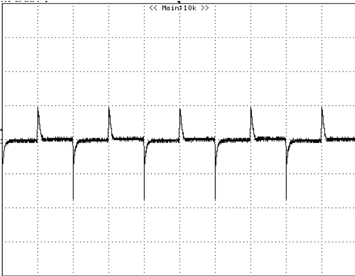
Figure 19: Typical transient response to step load change at 1A/\mu S from 100%~ 0%~100% of I_o , max at 12Vin, 1.2Vout (Cout = 1uF ceramic, 47uF+10uFceramic) CH1 : VOUT, 0.1V/div, 5mS/div
