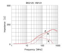
The data is reference only. Electrical characteristics vary depending on environment or measurement condition. TAIYO YUDEN reserves the right to make change to the Date at any time without notice. Before making final selection, please check product specification. 2013.07.26
